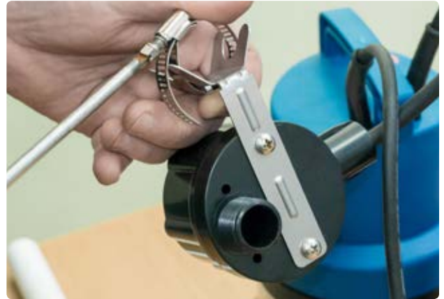
10. Adjust the hose clamp to fix the bar to the pressure PP pipe 25mm
