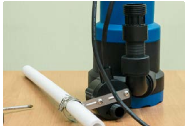
12. The clamp is not rigidly mounted, so that it can be adjusted further in future if necessary
