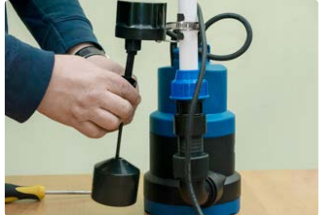
14. Fix the second part to the upper part of float switch
