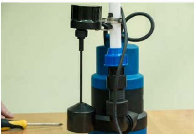
15. Adjust the height of float switch on the PP tube
