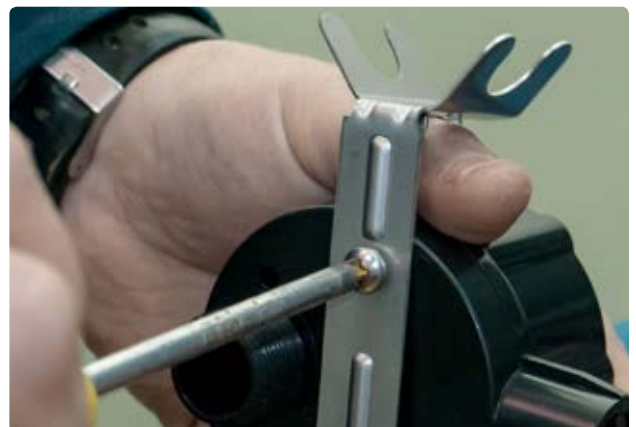
8. Fix the mounting plate on the upper part of float switch
