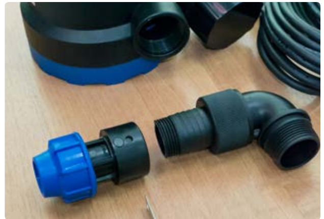
4. Put a nipple by twisting on the L-shaped connector
