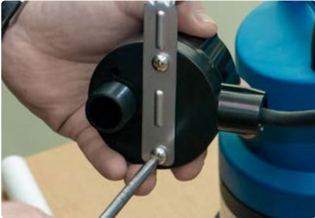
9. Fix the mounting plate with two screws
