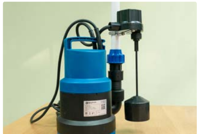
16. Float switch must neither touch pump nor water ejection unit
